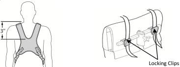
To free-up the user, simply release the quick-release buckles and bring the breastplate above the head toward the back of the wheelchair. When sitting the user, all the lower adjustments will have remained. Simply buckle the mechanism to retrieve prior configurations or make it tighter/looser depending on clothing and comfort.
