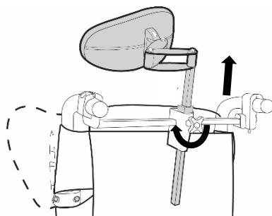
To pull out the headrest stem, use the lobe knob and turn **counter clockwise**.
