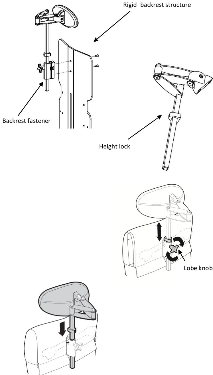
The SUMMUS headrest system is attached to the rigid backrest structure of FLEXUS.
