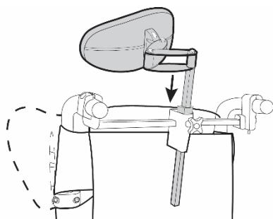
When reinstalling, use the cursor to guide you with the reinsertion of the mounting bar. Pull out the plunger, slide the bar into the anchor. Lock in place by push in the plunger.
