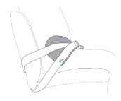
A 45° angle should be respected while assuring that the lateral pads remain flat on the iliac crests.
