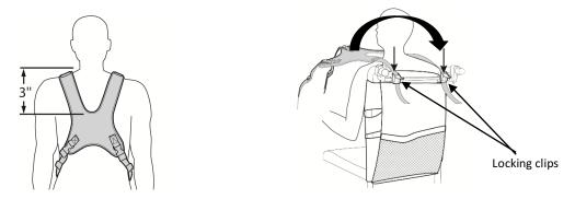
To free-up the user, simply release the quick-release buckles and bring the breastplate above the head toward the back of the wheelchair. When sitting the user, all the lower adjustments will have remained. Simply buckle the mechanism to retrieve prior configurations or make it tighter/looser depending on clothing and comfort.
