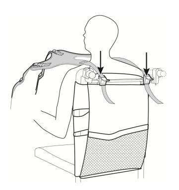
When it is time to sit user, reposition the mounting bar in a horizontal position and open the clips of both breastplate fasteners and insert upper straps through the clips.
