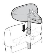
The SUMMUS headrest system is attached to the rigid backrest structure of FLEXUS.
