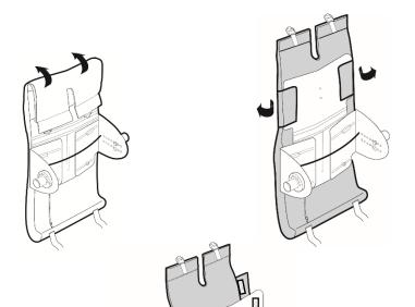
Lift the top flap to access the lateral fabric flaps located on either side of the backrest top.
