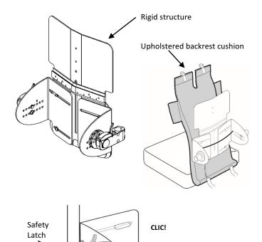
FLEXUS is made of a fully adjustable rigid structure (hardware) covered by an upholstered backrest cushion.
