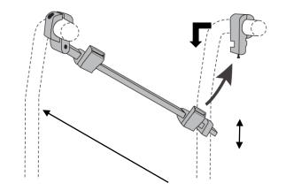
To fold the wheelchair, pull down the plunger, push forward and downward the mounting bar. It will come to a vertical position.
