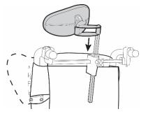
To pull out the headrest stem, use the lobe knob and turn **counter clockwise**. TO AVOID LOSING THE LOBE KNOB, always keep it screwed into the backrest fastener.
