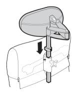
The SUMMUS headrest system is attached to the rigid backrest structure of FLEXUS.
