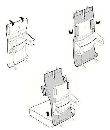
Lift the top flap to access the lateral fabric flaps located on either side of the backrest top.
