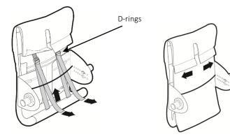
Before installing the upholstered backrest cushion, conduct a thorough check of all fasteners and secure any loose components following the required torque settings. IF YOU ARE UNCERTAIN ABOUT THE SAFETY, CONTACT IMMEDIATELY YOUR CLINICIAN / DEALER FOR ASSISTANCE.
