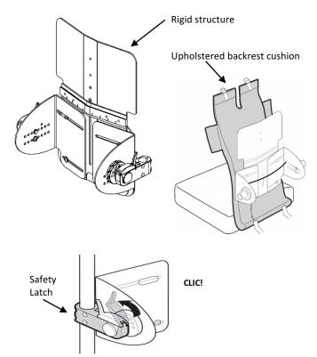
FLEXUS is made of a fully adjustable rigid structure (hardware) covered by an upholstered backrest cushion.
