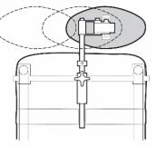
The flange bolt closest to the headrest cushion provides extra rotation for optimal posture of the head.
