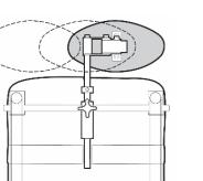
The flange bolt closest to the headrest cushion provides extra rotation for optimal posture of the head.
