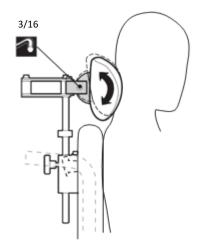
Slightly loosen the slant screw to change the headrest angle.
