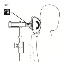
Slightly loosen the slant screw to change the headrest angle.
