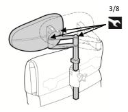
Slightly loosen the three (3) flange bolts to make multidirectional adjustments: front/back, lateral, rotational.
