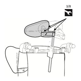
Slightly loosen the flange bolts to make multidirectional adjustments: front/back, lateral, rotational.
