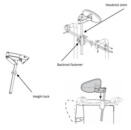
When using BACKUS & CURVUS backrests, SUMMUS is secured by a hardware system attached to the back canes of the wheelchair.
