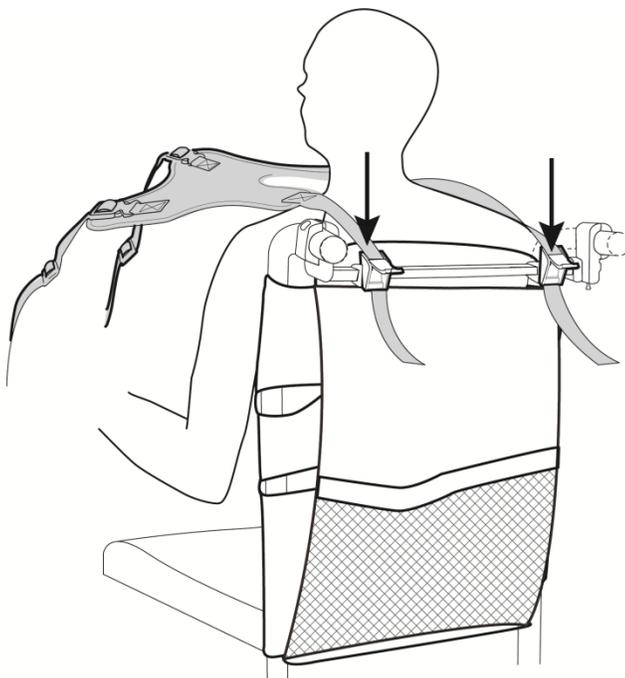
When it is time to sit user, reposition the mounting bar in a horizontal position and open the clips of both breastplate fasteners and insert upper straps through the clips.
