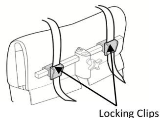
**To free-up the user, simply release the quick-release buckles and bring the breastplate above the head toward the back of the wheelchair. When sitting the user, all the lower adjustments will have remained. Simply buckle the mechanism to retrieve prior configurations or make it tighter/looser depending on clothing and comfort.**
