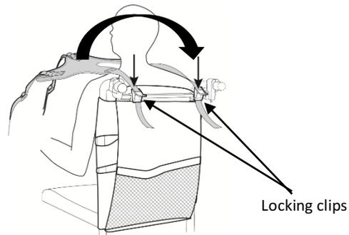
To free-up the user, simply release the quick-release buckles and bring the breastplate above the head toward the back of the wheelchair. When sitting the user, all the lower adjustments will have remained. Simply buckle the mechanism to retrieve prior configurations or make it tighter/looser depending on clothing and comfort.
