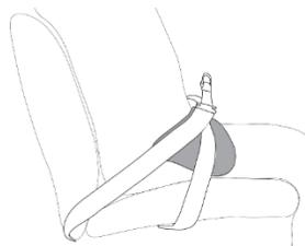
A 45° angle should be respected while assuring that the lateral pads remain flat on the upper portion of the thighs.
