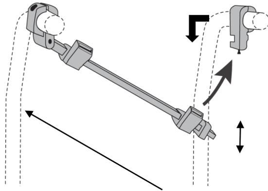
To fold the wheelchair, pull down the plunger, push forward and downward the mounting bar. It will come to a vertical position.
