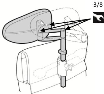
Slightly loosen the three (3) flange bolts to make multi-directional adjustments: front/back, lateral, rotational.
