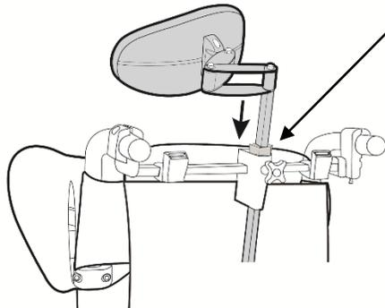
To memorize the desired height, a height lock is secured by tightening its socket set-screw.
