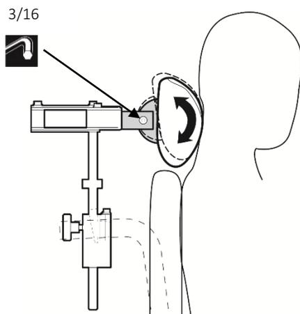
Slightly loosen the slant screw to change the headrest angle.
