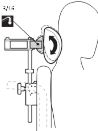
Slightly loosen the slant screw to change the headrest angle.
