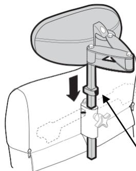
To memorize the desired height, a height lock is secured by tightening its socket set-screw.
